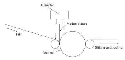
Fig. 7.14 Extrusion coating of plastic film.
