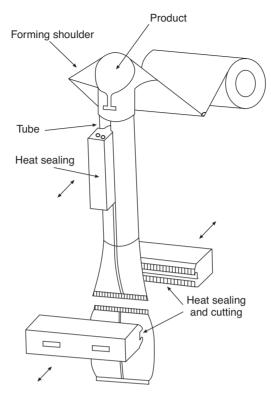
Fig. 7.6 Vertical form/fill/seal (f/f/s) machine.
