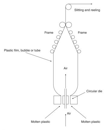
Fig. 7.3 Blown film manufacture.
