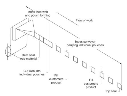
Fig. 7.5 Horizontal form/fill/seal sachet/pouch machine.
