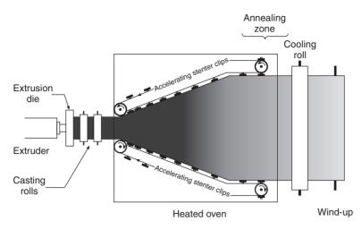
**Fig. 7.4** TD orientation by Steiner and MD orientation by acceleration in machine direction. (Courtesy of The Packaging Society.)
