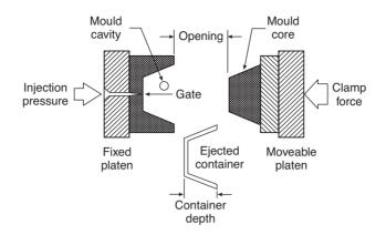
Fig. 7.11 Injection moulding. (Courtesy of The Packaging Society.)
