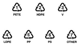
Fig. 7.16 Society of the plastics industry (SPI), resin identification codes.
