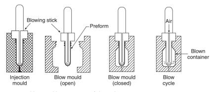
Fig. 7.9 Injection blow moulding. (Courtesy of The Packaging Society.)
