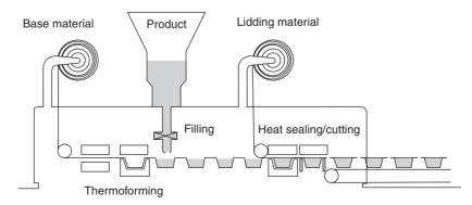
Fig. 7.12 Thermoforming, filling and sealing.
