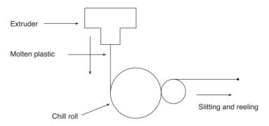
Fig. 7.2 Production of cast film.
