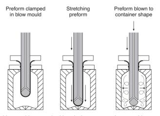
**Fig. 7.10** Stretch blow moulding – applicable to both extrusion and injection blow moulding. (Courtesy of The Packaging Society.)
