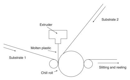
Fig. 7.15 Extrusion lamination.
