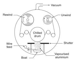
Fig. 7.13 Metallising process. (Courtesy of The Packaging Society.)
