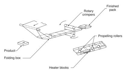
Fig. 7.7 Horizontal form/fill/seal (f/f/s), flowpack type machine.
